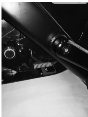
Figure 16. Studio 5 Cadence Sensor Mounting
