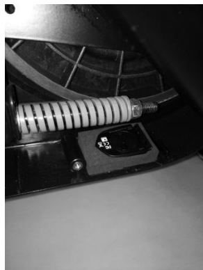
Figure 16. Studio 5 Cadence Sensor Mounting
