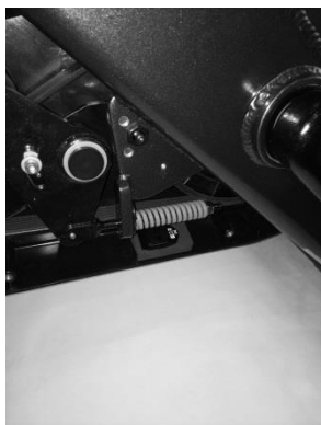
Figure 17. Studio 7 Cadence Sensor Mounting
